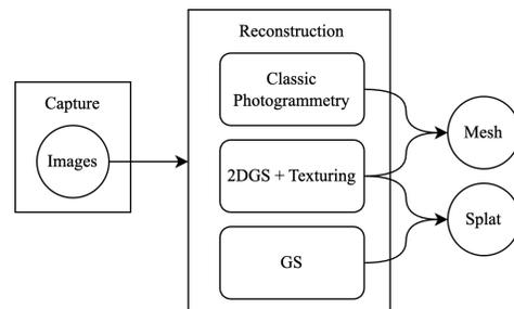
Fig. 1: The tested workflows rely on RGB images as input material and result in either splats or meshes as outputs.
